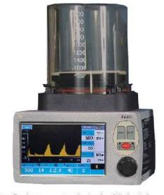
Battery Back-up Drive Gas 60 minutes (on full charge) Oxygen or Air (dry and oil free) at 45 to 100 psi (310 to 689 kPa)
